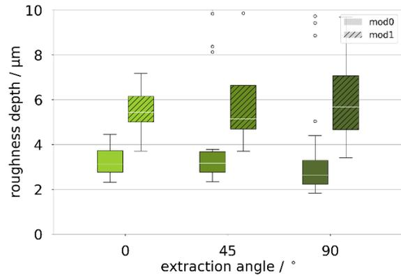
**Fig. 4.** average roughness and roughness depth for the milled surface of BZ6 test specimens.
