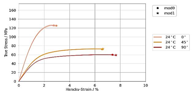
**Fig. 5.** force – displacement – diagram and true stress – strain – diagram of smooth (mod0) and rough (mod1) specimens at room temperature for different extraction angles.
