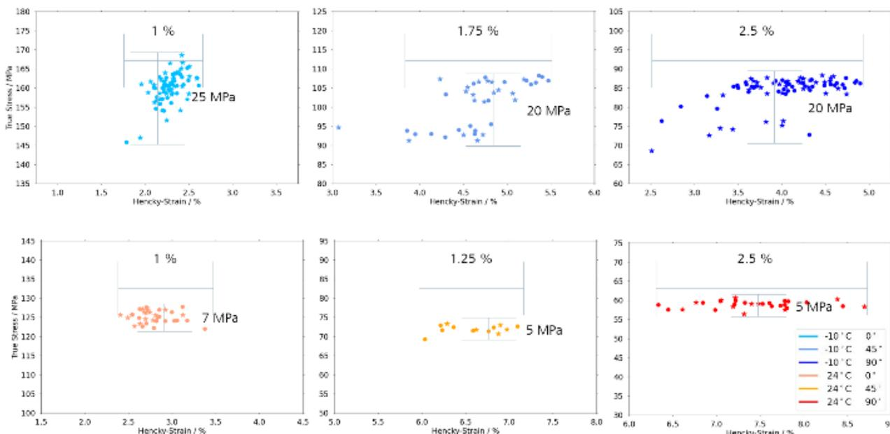
**Fig. 7.** True failure stress – failure strain – diagram of smooth (mod0) and rough (mod1) specimens at -10 °C and 24 °C for different extraction angles with indicated scatter band.
