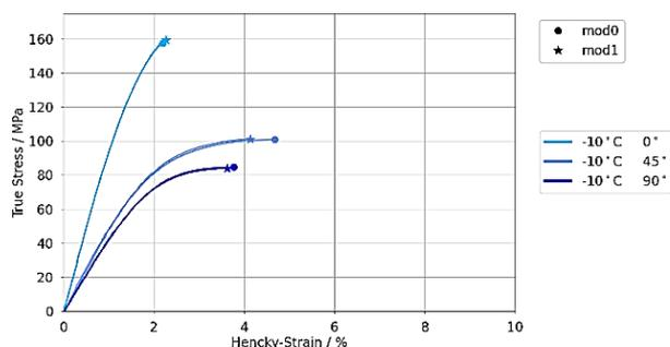
**Fig. 6.** true stress – strain – diagram of smooth (mod0) and rough (mod1) specimens at -10 °C for different extraction angles.
