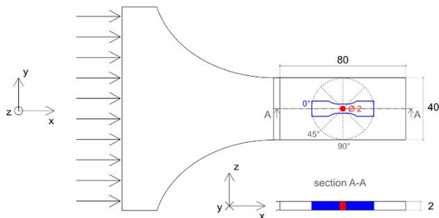
**Fig. 2.** Geometry of the novel plate to extract BZ6 specimens (blue) for tensile tests. Centric position of microcomputer tomography specimen (red).
