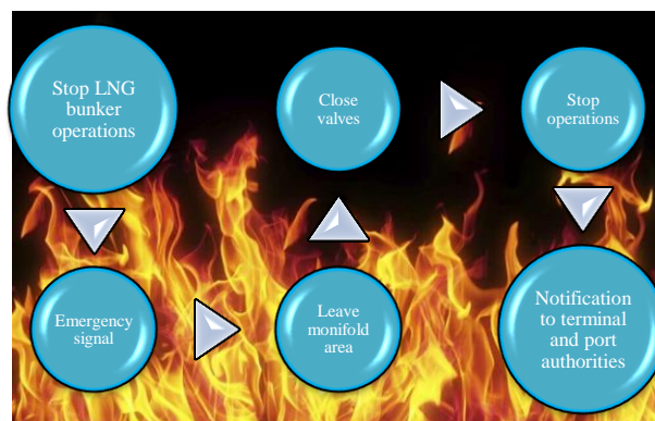
Fig. 3. Procedure in case of fire on board.
