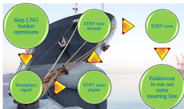
Fig. 6. Procedure in case of Mooring line failure.
