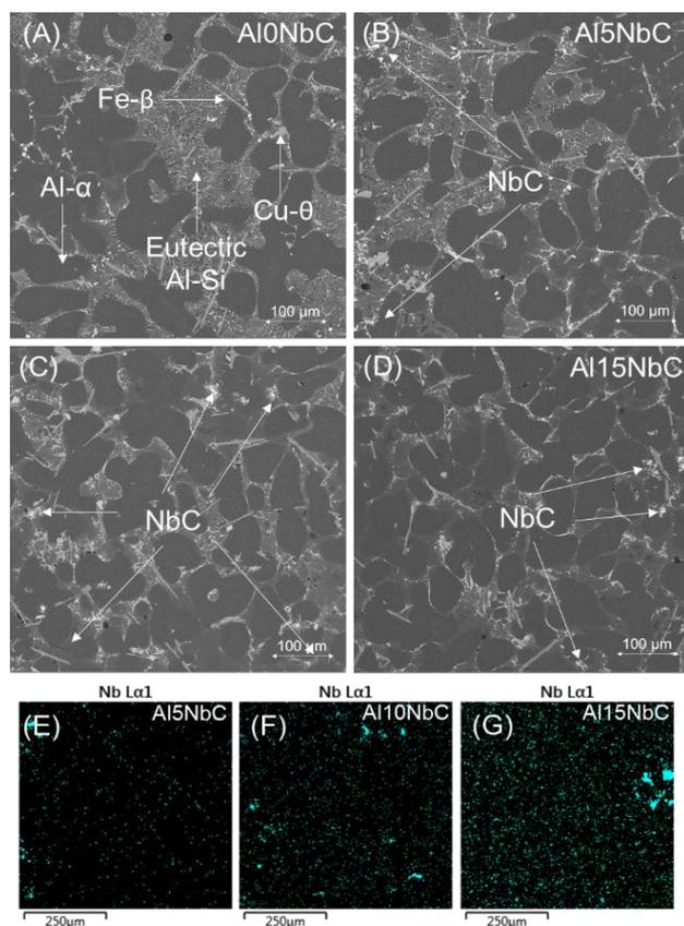
**Fig. 1.** SEM images after partial remelting samples showing the NbC particles in (A) Al0NbC (B) Al5NbC (C) Al10NbC (D) Al15NbC, and EDS maps of Nb from (E) Al5NbC, (F) Al10NbC, (G) Al15NbC
