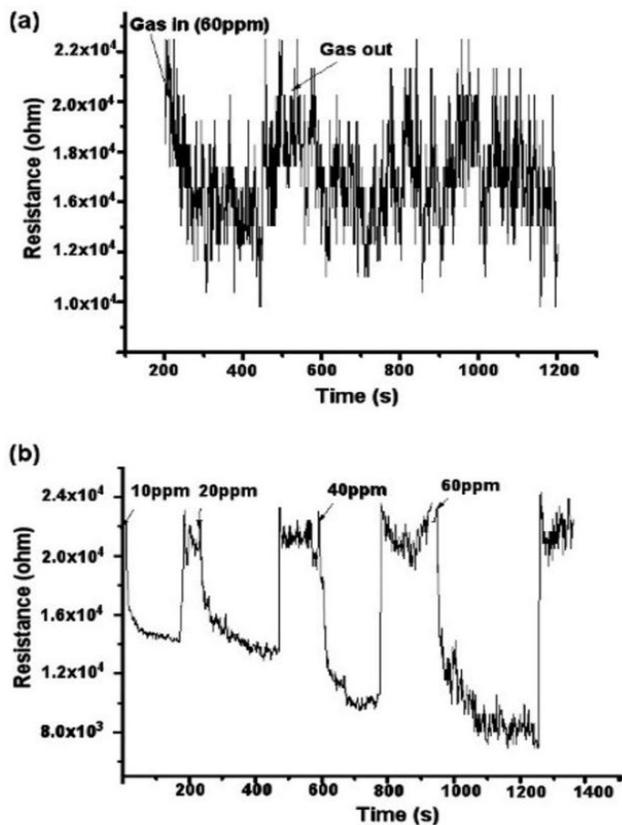
Fig. 5: Dynamic gas response for acetone of (a) PANI/Mn<sub>3</sub>O<sub>4</sub> (1 mM) and (b) PANI/Mn<sub>3</sub>O<sub>4</sub> (3 mM).
