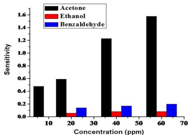
Fig. 6: Sensitivity of PANI/Mn<sub>3</sub>O<sub>4</sub> towards acetone, benzaldehyde dan ethanol.
