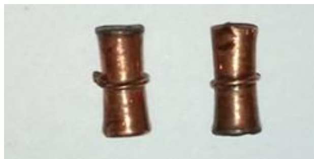
Fig. 5. Electroplated cylindrical ABS part using chromic acid for etching.
