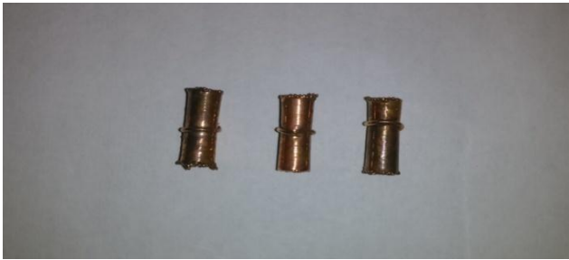
Fig. 6. Electroplated cylindrical ABS part using aluminium charcoal paste.
