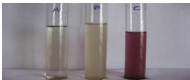
Fig. 2 Tube A- Auric acid, Tube B- Plants extract, Tube C- Green gold nanoparticle solution.
