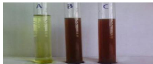
Fig. 1 Tube A- Auric acid, Tube B-Fruit Extract, Tube C- Green gold nanoparticles solution.
