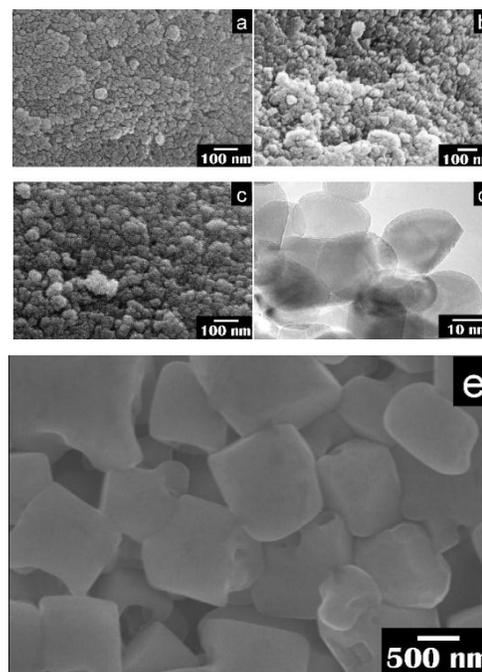
**Fig. 4.** FESEM image of the as prepared NiO/YSZ calcined at (a) 400°C, (b) 500°C, (c) 600°C, along with (d) TEM image the as prepared NiO/YSZ calcined at 600°C, and (e) the NiO/YSZ sintered anode at 1350°C (before reduction).
