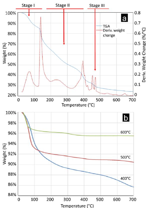
**Fig. 1** TGA spectra of (a) dried Ni/Zr/Y/alginate beads before calcination; and (b) the as prepared NiO/YSZ after calcination (at 400, 500, and 600°C for 6h)
