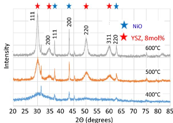
**Fig. 2.** XRD pattern of the as prepared NiO/YSZ powders calcined at 400, 500, and 600°C for 6h.
