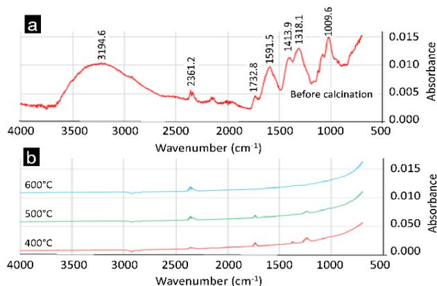
**Fig. 3.** FTIR spectra of (a) the dried Ni/Zr/Y/alginate beads before calcination; and (b) the as prepared NiO/YSZ after calcination (at 400, 500, and 600°C for 6h).
