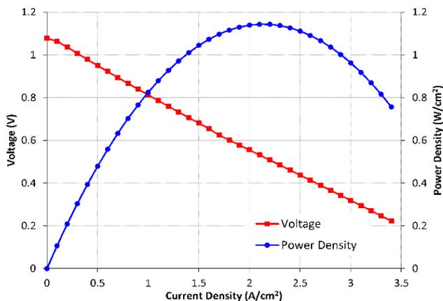
**Fig. 5.** Electrochemical performance of the anode-supported cell measured at 850°C under flowing a humidified hydrogen gas flowing at 20 ml/min.
