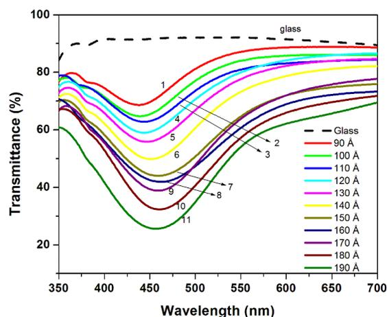
Fig. 2. Transmittance of plain glass (dotted line) and 1D-PBG coated glass with varying thickness of Ag (90 Å - 190 Å).
