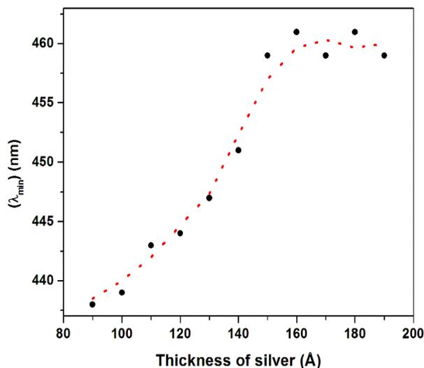
**Fig. 3.**  $\lambda_{\min}$  (nm) versus thickness of Ag (90 Å - 190 Å).
