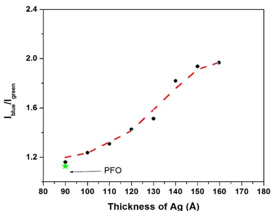
Fig. 5. Blue to green peak intensity ratio ( $I_{blue}/I_{green}$ ) with varying thickness of Ag.
