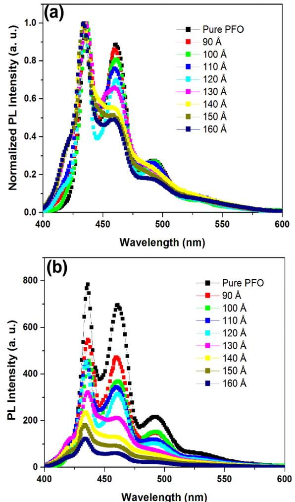
**Fig. 4.** (a) Normalized photoluminescence and (b) photoluminescence spectra of PFO coated over plain glass and 1D-PBG coated glass.
