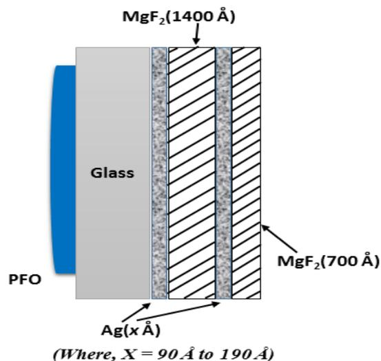
Fig. 1. Schematic diagram of PBG on one side of glass substrate and PFO on the other side.
