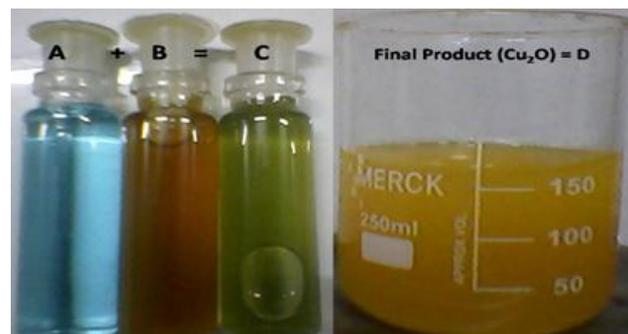
Fig. 2. It is a reaction, (A) illustrate  $\text{CuSO}_4 \cdot 5\text{H}_2\text{O}$  (B) Carrot waste extract (C) Mix up A and B and (D)  $\text{Cu}_2\text{O}$  HMs after reduction.
