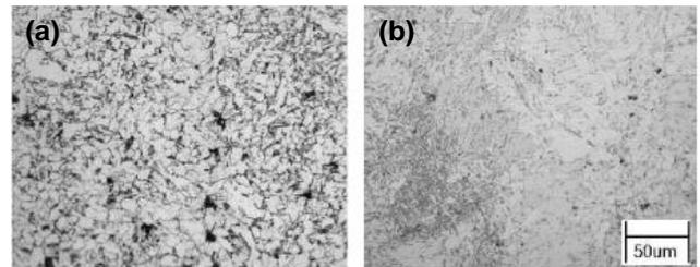
Fig. 4. Optical Microscope photos show the microstructure comparison between a) steel S4 contains 0.8% Ni, and b) S1 without Ni.
