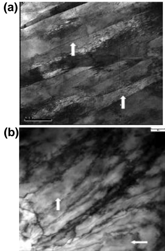
Fig. 5 TEM micrograph shows the effect of Ni additions on acicular ferrite morphology in a) steel S4 has 0.8% Ni, and b) S1 without Ni.
