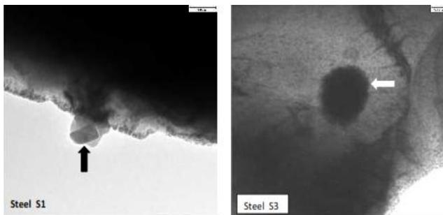
Fig. 3. TEM photo shows the Ti oxides in steel S1 and S3.
