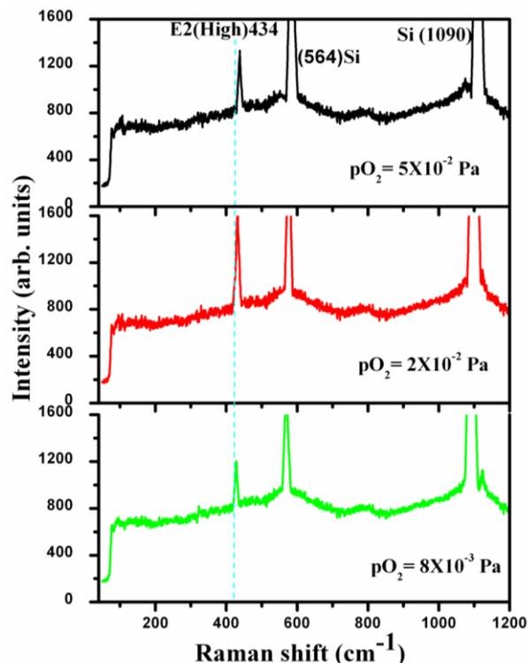
Fig. 6. Raman spectra of ZnO films at different oxygen partial pressures.
