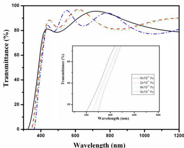
Fig.7. Optical transmittance spectra of ZnO films at different oxygen partial pressures.
