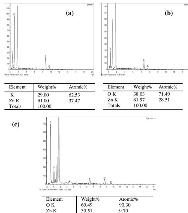
**Fig. 3.** EDS spectra of ZnO films (a)  $5 \times 10^{-3}$  Pa (b)  $2 \times 10^{-2}$  Pa (c)  $5 \times 10^{-2}$  Pa.
