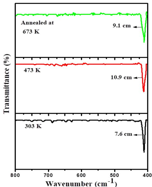
**Fig. 10.** FTIR spectra of ZnO films at different annealing temperatures.
