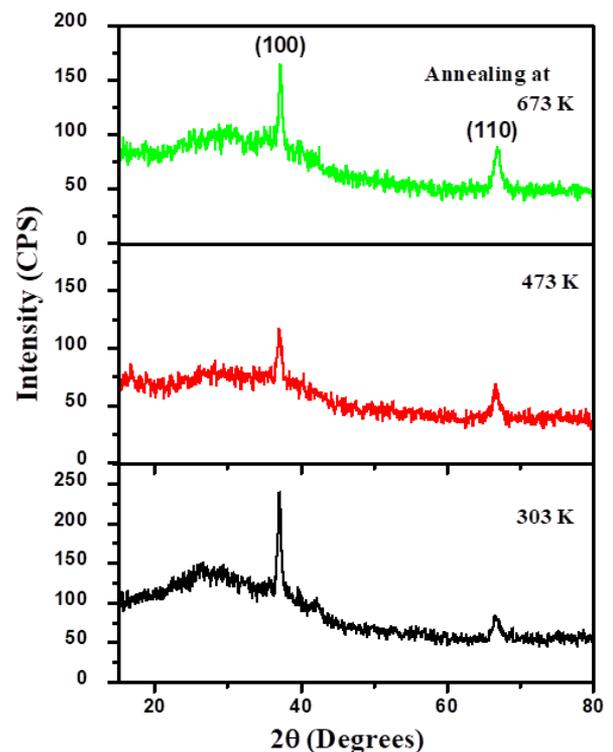
Fig. 8. XRD patterns of ZnO films deposited at various annealing temperatures.
