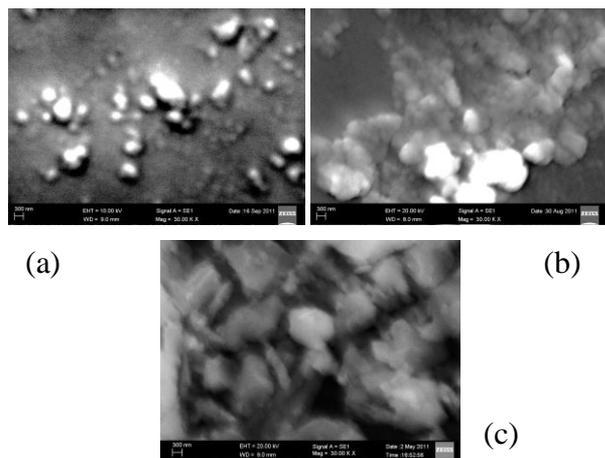
**Fig. 9.** SEM images of ZnO films (a) 303 (b) annealed at 473 K (c) annealed at 673 K.
