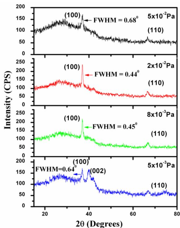
**Fig. 1.** XRD patterns of ZnO films deposited at various oxygen partial pressures.
