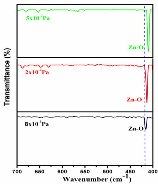
Fig. 5. FTIR spectra ZnO films at (a)  $5 \times 10^{-2}$  Pa (b)  $2 \times 10^{-2}$  Pa (c)  $8 \times 10^{-3}$  Pa.
