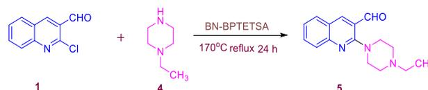
**Scheme 3.** Synthesis of 2-(4-ethylpiperazin-1-yl) quinoline-3-carbaldehyde.
