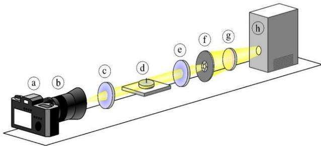
**Fig. 2.** Scheme of optical set using for contact angle measurement, from left: a) digital camera, b) zoom lens ( $f = 300$  mm), c) convex lens ( $f = 50$  mm), d) fiber submerged into the water, e) convex lens ( $f = 50$  mm), f) circular aperture, g) light diffuser, h) light source.
