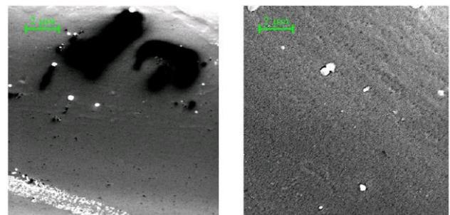
**Fig. 5.** SEM images of reference (left) and 240 seconds plasma treated (right) fibers.
