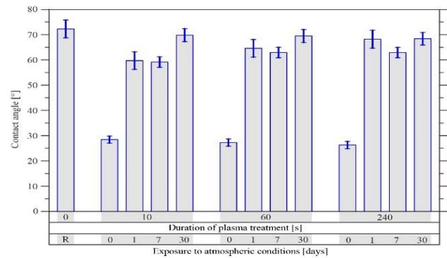
**Fig. 4.** Contact angles depending on the plasma treatment time and the exposition to atmospheric conditions measured on fibers.
