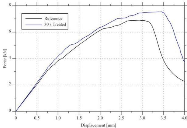
**Fig. 6.** Force-displacement diagram of cement samples reinforced with reference and 30 seconds plasma treated fibers.
