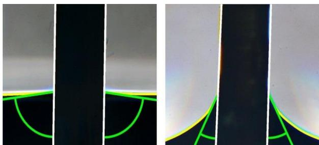
**Fig. 3.** Reference (left) and treated (right) fiber submerged into the water with outlined contours.
