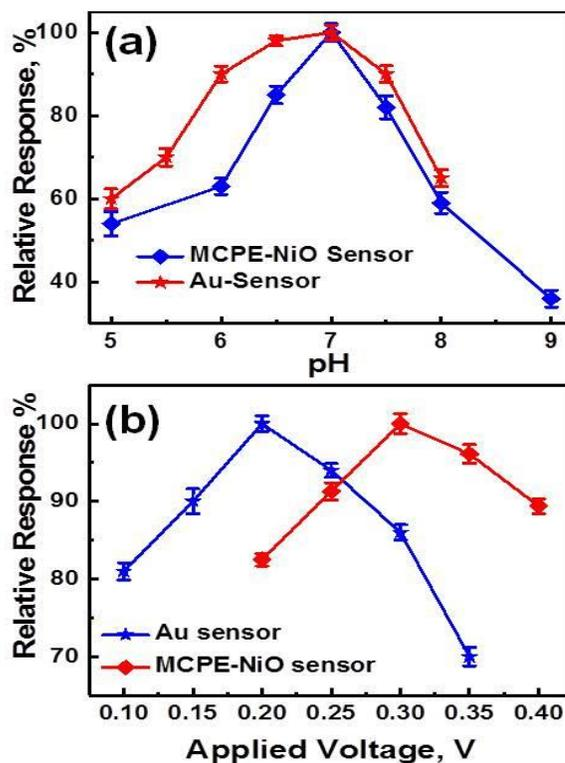
**Fig. 4.** Effect of solution pH (a) and applied potential (b) on the steady-state current response of MCPE-NiO-Lac and Au-Lac electrode of Clark type DO sensor in 0.2 M PBS solution containing 1 mM catechol.
