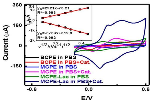
**Fig. 2.** Cyclic voltammograms of BCPE, MCPE-NiO, MCPE-NiO-Lac in 0.2 M pH 7 PBS buffer solution containing 1mM catechol at a scan rate of  $50 \text{ mV s}^{-1}$ . Inset picture shows the linear variation of the peak current as a function of the square root of the scan rate for MCPE-NiO electrodes.
