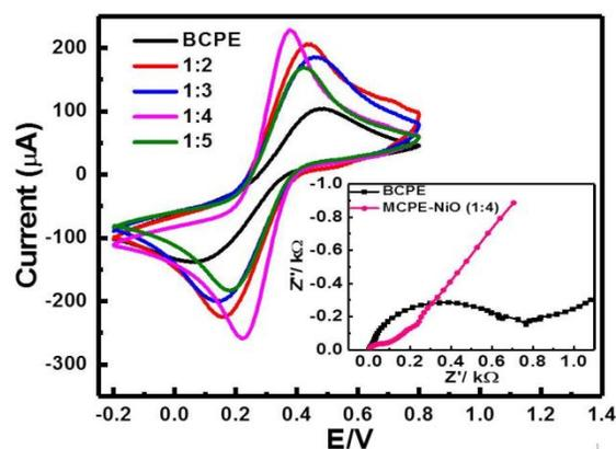
**Fig. 1.** CVs of 10 mmol L<sup>-1</sup>  $Fe(CN)_6^{3-/4-}$  on various MCPE-NiO electrodes prepared with the mass ratio of NiO NCs to graphite powder as 1:2, 1:3, 1:4, and 1:5 at a scan rate of 50 mVs<sup>-1</sup>. Inset picture gives EIS spectra of BCPE and MCPE-NiO (1:4) performed in 0.1M KCl and 10 mM  $Fe(CN)_6^{3-/4-}$  solution.
