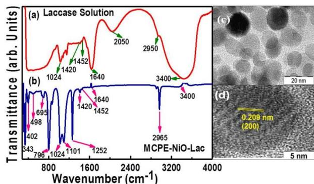
**Fig. 3.** FTIR spectra of (a) laccase solution (b) laccase immobilized NiO NCs-carbon paste. (c) TEM image of NiO particles in carbon paste and (d) HRTEM of the NiO nanocrystal imaged along (200) crystal plane.
