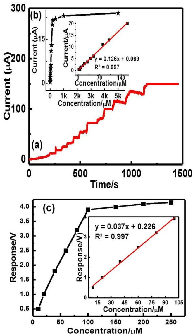
**Fig. 5.** (a) Chronoamperometric response of MCPE-NiO-Lac on successive addition of different concentration and volume of catechol solutions into pH=7, 0.2 M PBS solution at an applied potential of 0.3V; (b) Calibration curve with fitting for MCPE-NiO-Lac electrode. Inset: Calibration curve showing linear fitting in the range 0-150  $\mu\text{M}$ ; (c) Calibration curve with fitting for Au-Lac electrode. Inset: Calibration curve with linear fitting in the range 0-100  $\mu\text{M}$ .
