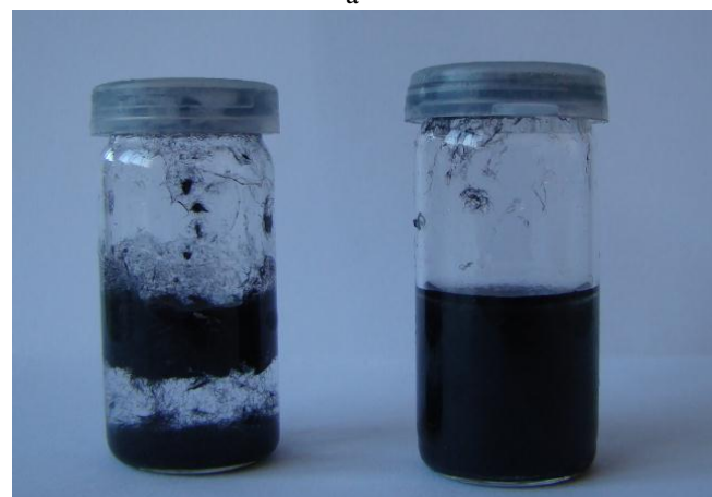
Fig. 1. SEM of carbon microfibers (a) and dispersion of unmodified (left-hand side) and modified (right-hand side) carbon microfibers in water.
