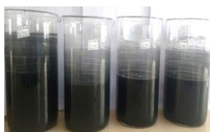
Fig. 6i. With 0.05% surfactant 60 after preparation.
