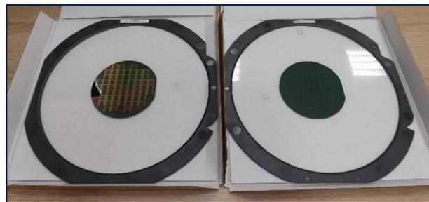
**Fig. 12.** Silicon wafers with electrochemical microchips.
