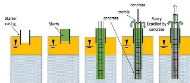
Fig. 1. Steps in the construction of drilled shafts [6].
