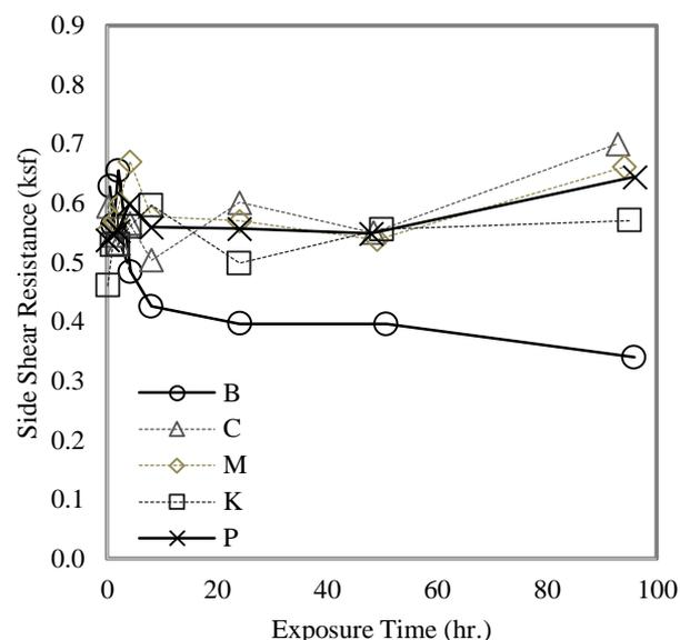
Fig. 4. Performance of polymer (CKM) and mineral slurry (B).
