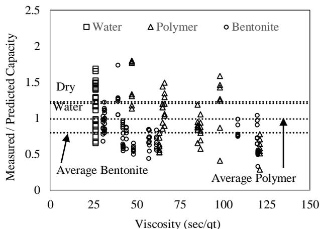
Fig. 5. Strength ratio versus slurry viscosity.
