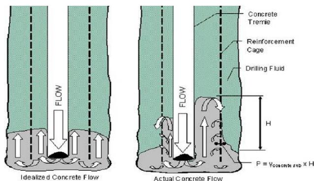
Fig. 2. Idealized and actual concrete flow patterns.
