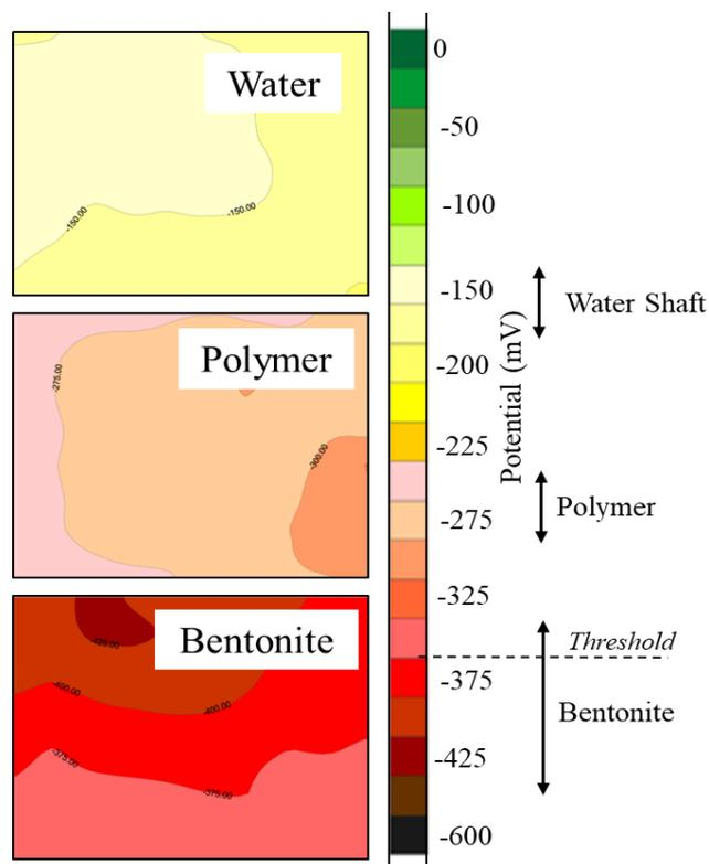
Fig. 6. Surface potential measurements (below -350 is corroding).
