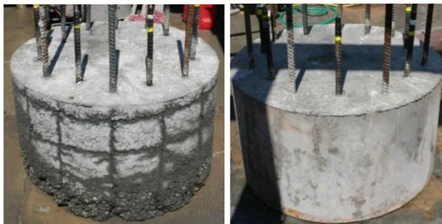
Fig. 3. Rebar pullout specimens: bentonite (left), polymer (right).
