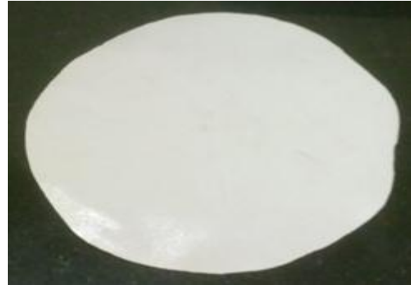
Fig. 1 PVDF-PZT composite film prepared by solvent casting followed by hot pressing
