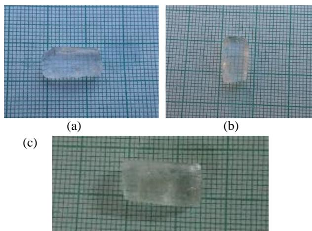
**Fig. 1.** (a) As grown Mannitol single; (b) Irradiated (2 kGy dose) Mannitol crystal single crystal; (c) Irradiated (4 kGy dose) Mannitol single crystal.
