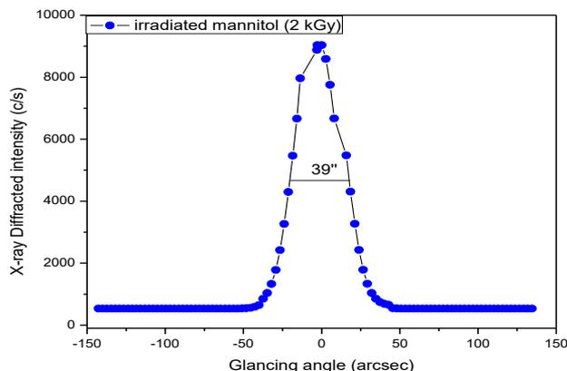
Fig. 4. HRXRD curve for irradiated Mannitol single crystal.
