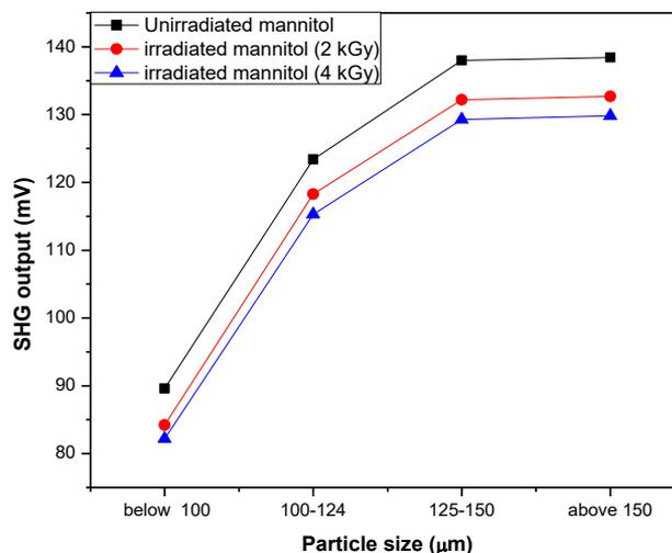
Fig. 6. SHG intensity versus particle sizes for pure and irradiated Mannitol single crystal.
