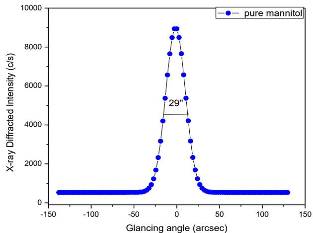
**Fig. 3.** HRXRD curve for pure (2 kGy) Mannitol single crystal.
