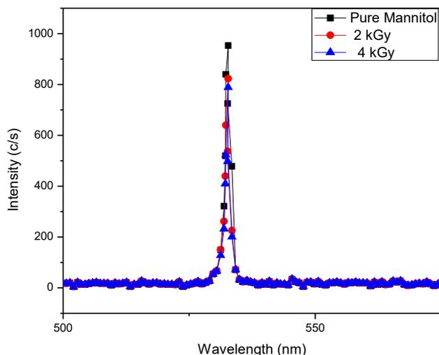
Fig. 7. SHG intensity for pure and irradiated Mannitol single crystal.
