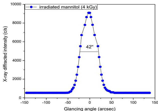
Fig. 5. HRXRD curve for irradiated (4 kGy) Mannitol single crystal.
