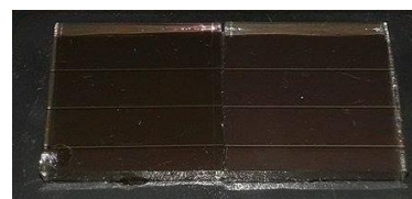
Current and near future papers distribution on the perovskite solar cells per year and type, and photo of perovskite solar cell laboratory sample produced at the Department of Microelectronics, TU-Sofia.
